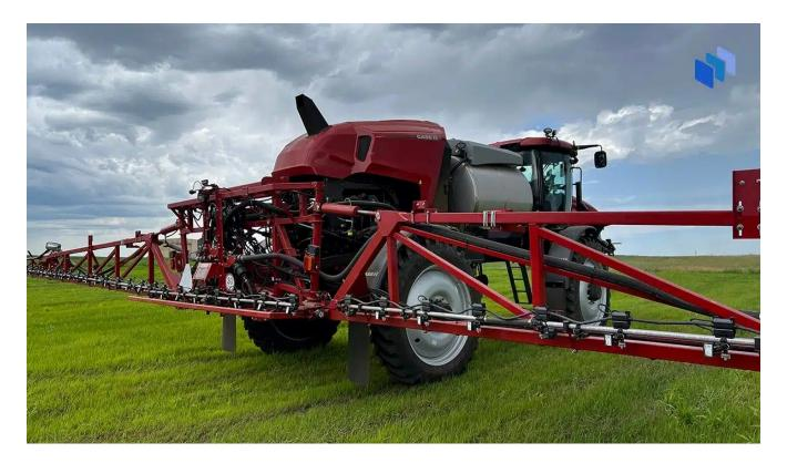
We also saw an existing, highly automated crop sprayer that used AI to improve one of the more challenging tasks in farming. While the base machine can already adjust how spray is used based on factors like speed and turning, an Augmenta machine learning sensor array makes it decidedly smarter. It can stop spraying when it sees an empty field ahead, and self-drive on very precise lines that keep it from running over crops. Radar even corrects the spray for the booms as they wobble.
