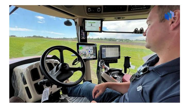
There's a host of information in the cockpit, too. A combination of camera data and positioning can show just which areas you've already covered. You can see just which nozzles are spraying and to what degree.
