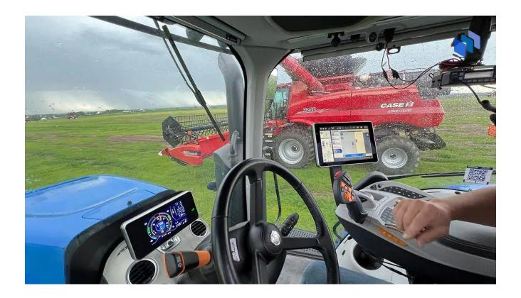
The last demo we saw was also for in-use tech. It's a semi-autonomous cart system that syncs a tractor (carrying the cart) with the combine that wants to unload the grains it's collecting.
